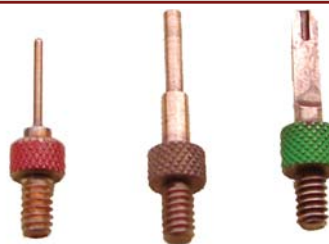
Extraction Tools 115-0150-000, Socket contact extractor (from front of plug) 115-0392-000, Pin contact extractor (from front of receptacle) 115-0147-000, Insertion (from rear) both pin and socket
